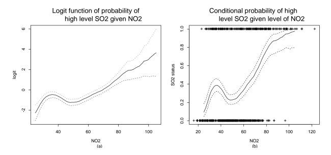
Figure 7: Logistic regression of the status of high level  $SO_2$  on the level of  $NO_2$ . (a) Estimated logit function of the conditional probability. (b) Estimated probability function and observed data.
