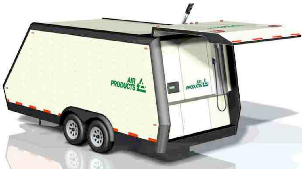
Figure 6: Mobile Hydrogen Refueling Unit
