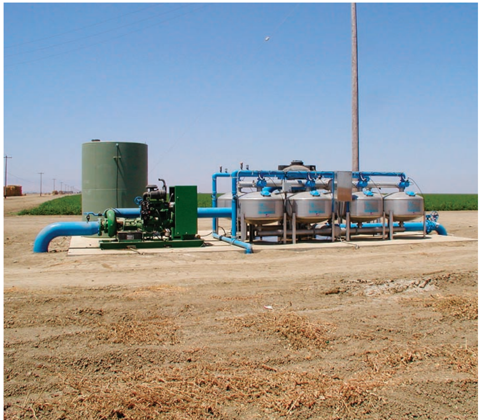
To minimize the uptake of shallow, saline groundwater — which can affect tomato yields — sufficient irrigation water must be applied in the root zone to ensure adequate leaching. Above, filters, pumps and fertilizer tanks are part of drip irrigation systems.
