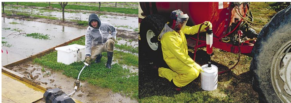
Left, former UC Davis graduate student Till Angermann monitors an autosampler to test the effects of best management practices for reducing dormant-season organophosphate runoff from orchard crops. Right, closed loading systems are important when handling certain organophosphate insecticides.
