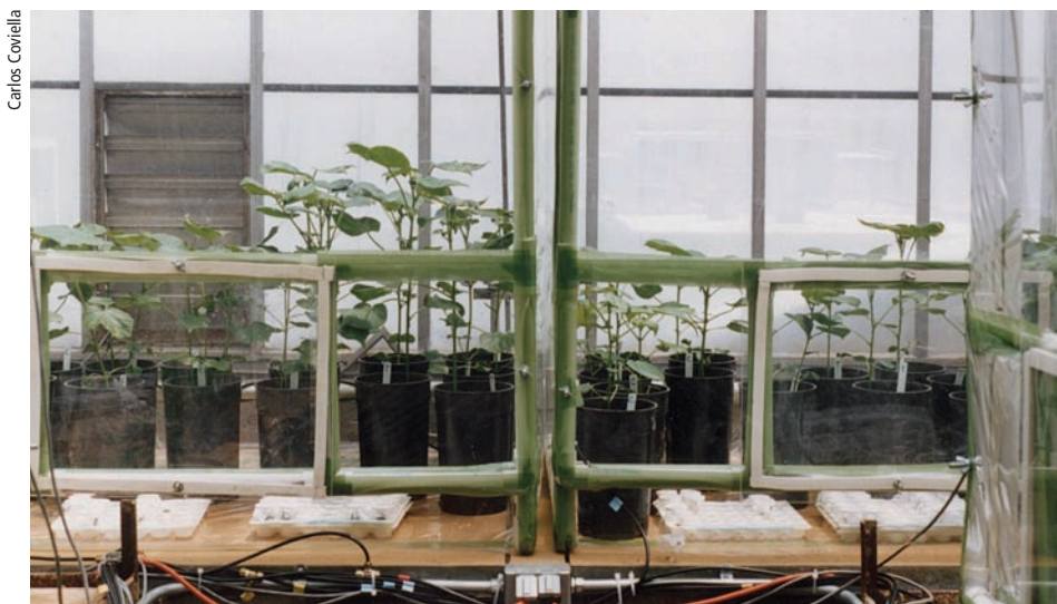
Plants grown at elevated carbon dioxide have lower nitrogen levels in the leaves, so insects must eat more to get the same amount of nutrient. In this chamber study, insects eating plants treated with Bacillus thuringiensis received a higher dose of the toxin as well, and died at significantly higher rates.
