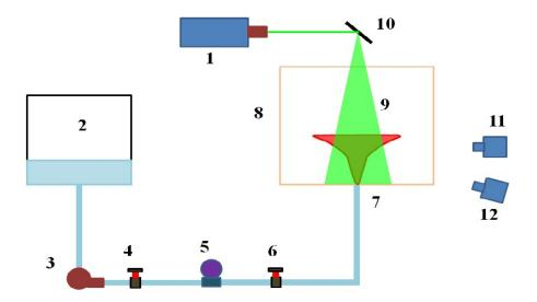
Figure 1: Schematic of experimental setup. 1. Laser source, 2.Tank (T1), 3. Centrifugal pump, 4,6.Control valve, 7. Jet nozzle, 8.Experimental tank (T2), 9. Laser sheet, 10. Mirror, 11. PIV camera, 12. PLIF camera.
