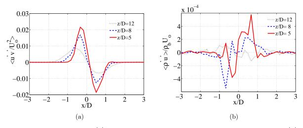
Figure 5: (a): Variation of  $< u^{'}v^{'}>$  for the different downstream location. (b): Variation of  $< \rho^{'}u^{'}>$  for the different downstream location.
