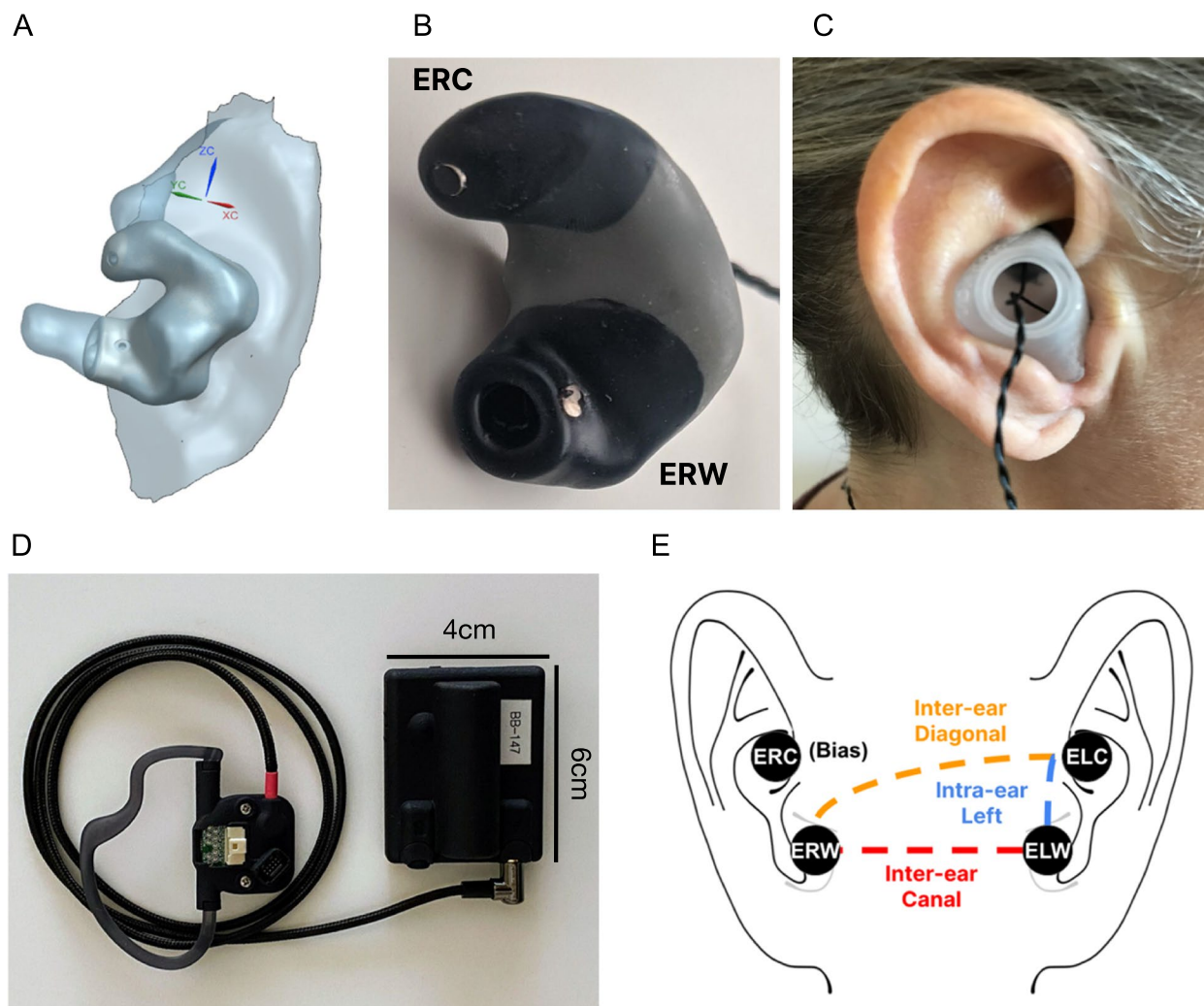
Fig. 1 Ear-EEG system. a 3D anatomical ear model obtained through optical ear scan. b A custom-made earbud with two electrodes per ear – Ear Right Cymba (ERC) placed in the cymba conchae and Ear Right Whole Canal (ERW) placed in the canal. c Non-invasive in-ear fit of the earbud. d Data acquisition system consists of the “earboard” (left) hooked around the left ear and a data recording device (right). e The electrodes’ placement, bipolar channel configuration, and naming convention
