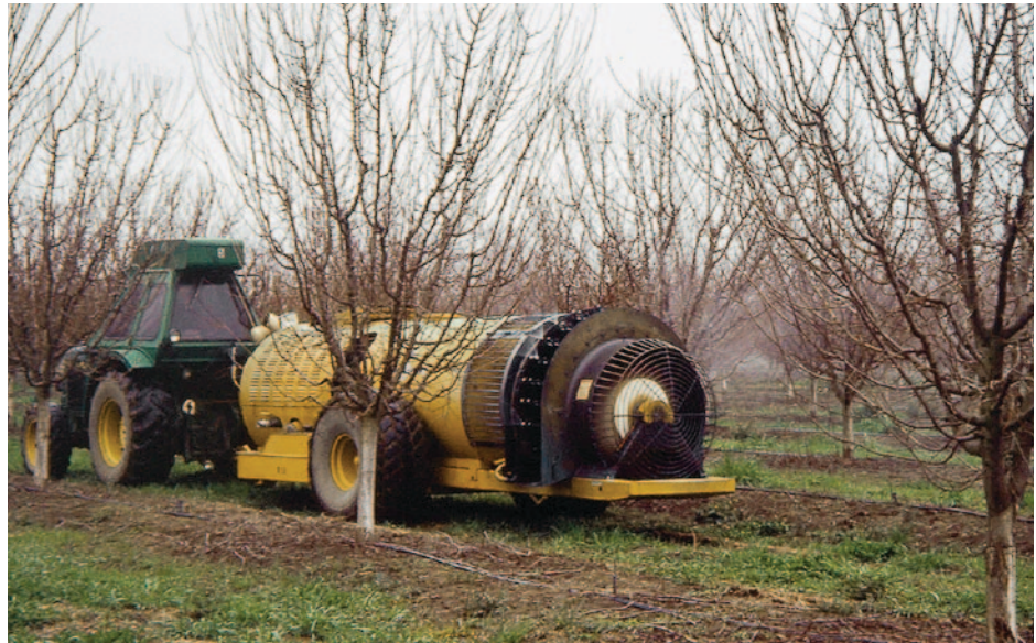
A commercial sprayer retrofitted with a target-sensing spray system applies dormant spray in a prune orchard near Chico. These "smart" systems only apply sprays where a tree is detected.
