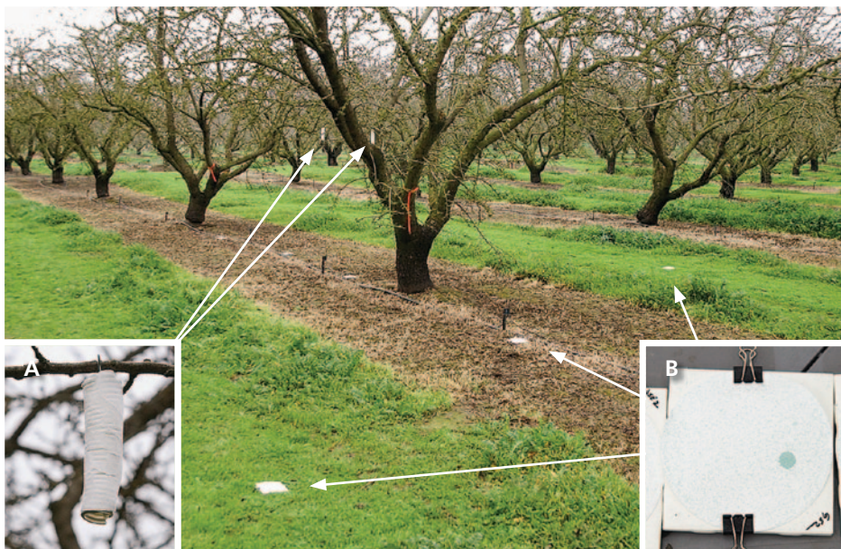
To monitor the tree and ground deposition of spray applications, (A) 1-inch-diameter cylinders fitted with fiber filters were suspended from almond trees at different heights and (B) 4.25-inch glass filters supported by flat ceramic tiles were laid on the orchard floor.
