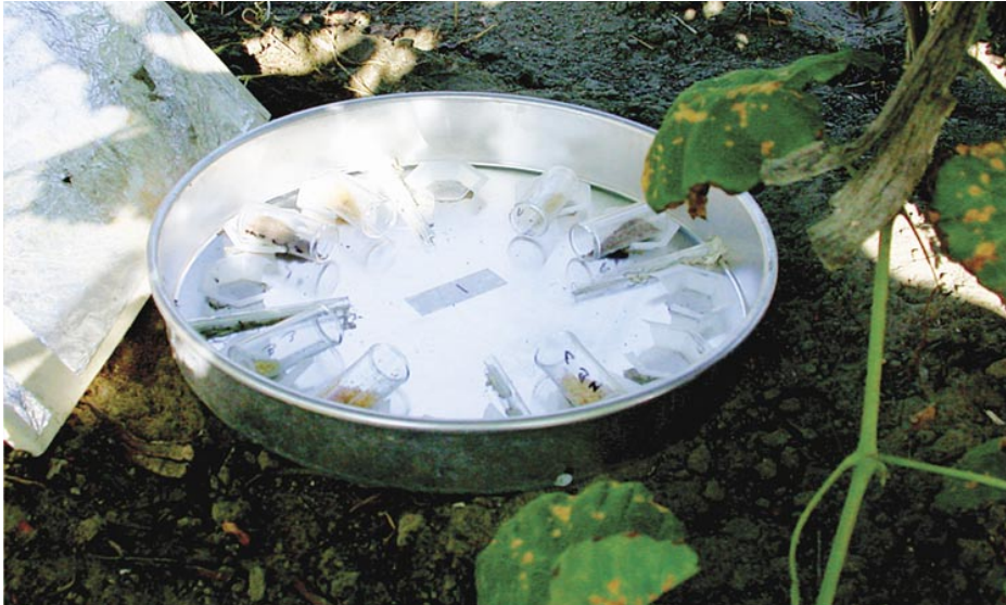
A choice-test arena (without lid) is used to determine the bait preferences of field ants.
