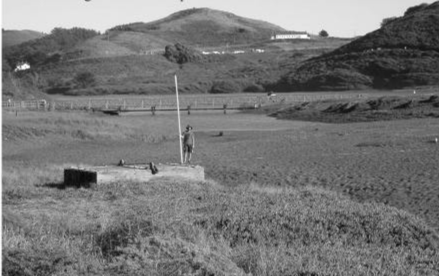
Dave Shaw holding surveying rod for first cross section (bridge over inlet channel in the background, military foundation remnant in the foreground). Depressed remains of inlet channel evident to the left of Dave and winding towards the right-front of the picture.
