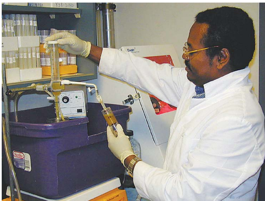
Compared with laborious and expensive in vivo testing, the in vitro gas production method provides a quick and easy way to calculate organic matter digestibility, quantify the energy value of feed mixtures and monitor microbial change in the rumen. Left , Girma Getachew fills syringes with buffered rumen fluid.
