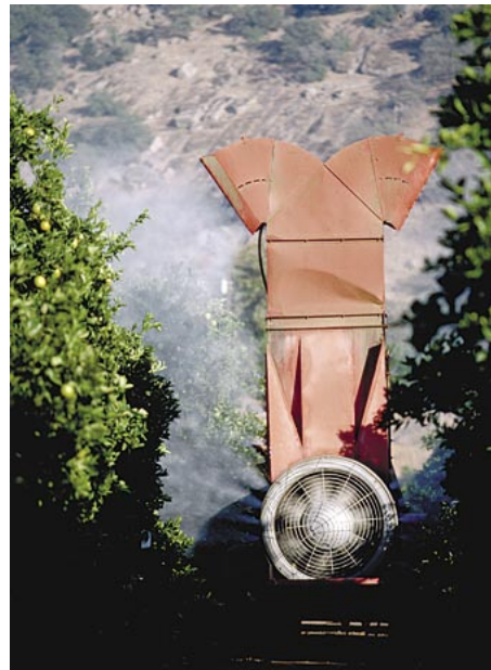
Above, in 1915 a worker sprayed dry sulphur on young prune trees infected with brown mite near Yuba City. Today, sulfur is still widely used as a pesticide to control mites on grapes, citrus and other crops. Right, an air-blast sprayer with tower treats citrus crops with petroleum-based oils to control citrus red mite and California red scale.
