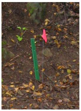
Sample three-foot aluminum post at cross-section location. Photo: TG 4/20/06
