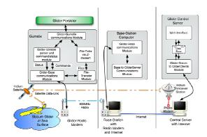
Block Diagram of Communication system for Gliders
