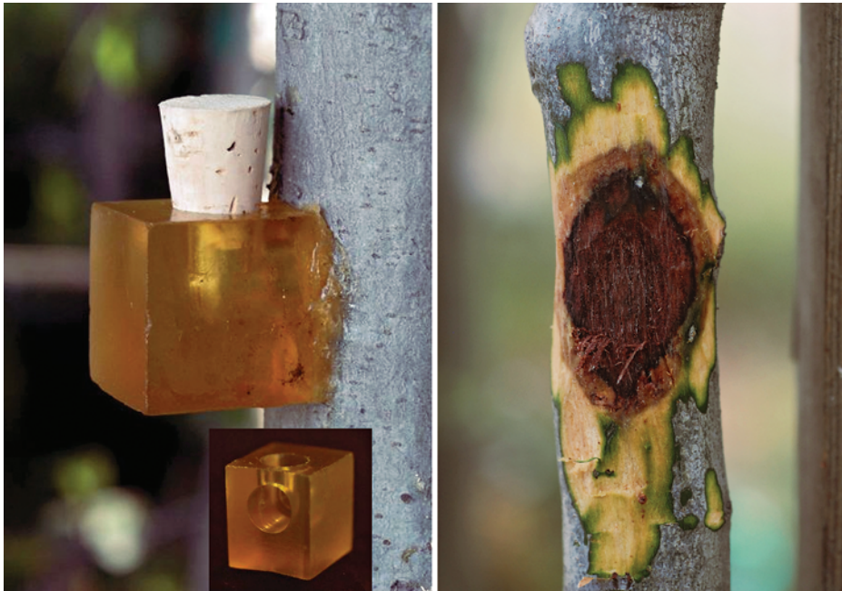
A plastic device developed at UC Berkeley is used to artificially infect trees with zoospores of P. ramorum .
