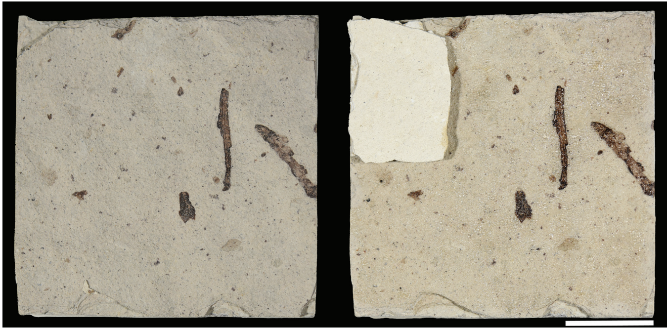
FIGURE 21. 1PB1 sample pre-treatment and just after treatment with PaleoBond PB40. The ethyl cyanoacrylate increases the contrast between the fossil inclusions and the paper shale matrix while also creating surface sparkles. Scale is 1 cm.
