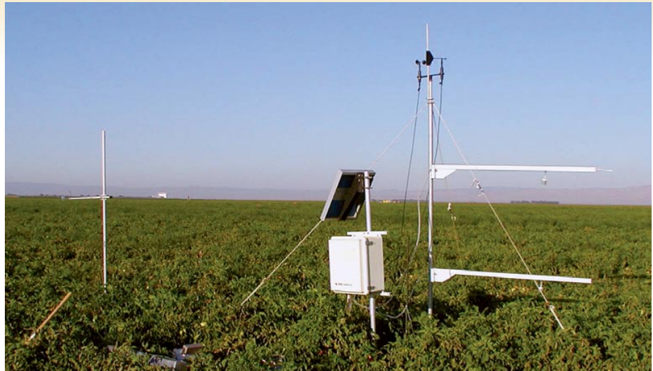
Thanks to site-specific breeding, processing tomato yields in California have increased by more than 50% since the early 1970s, while water-use efficiency has increased about 40%. Bowen ratio instruments were used to collect climate and soil data from processing tomatoes, in order to calculate evapotranspiration and update crop coefficients.
