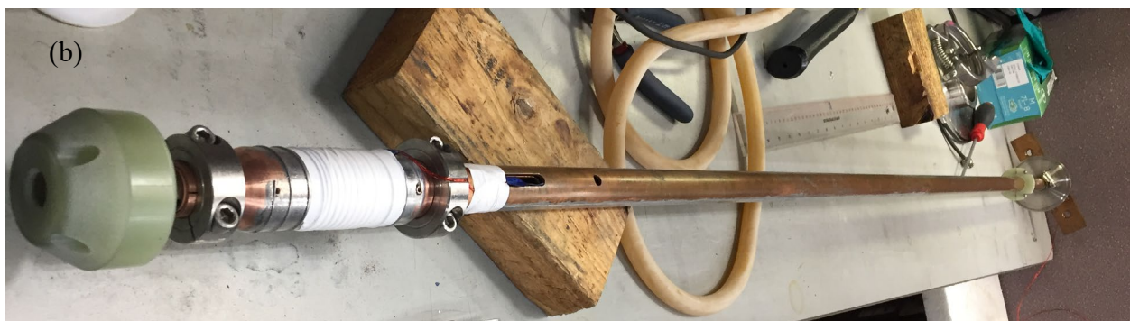
Figure 1 (a) Sample wire wound on the test mandrel which consists of a titanium barrel (black in the middle) and copper terminals. (b) The sample mounted on the test probe. A pair of voltage taps was soldered spanning 50 cm of sample length. The pressure contacts between the sample and the probe were made by two stainless-steel collar clamps.
