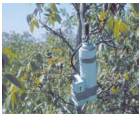
Pheromones can be applied in aerosol form, such as this experimental microsprayer, or "puffer," which releases precise doses at timed intervals.
