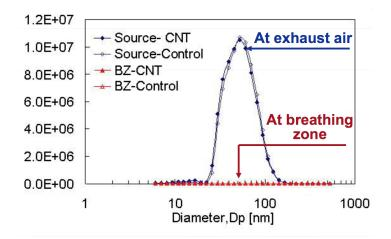
*Figure 12: Demonstration of the effectiveness of a fume hood at preventing exposure to carbon nanotubes*<sup>117-119</sup>.
