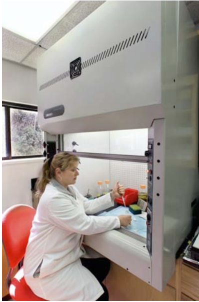
Figure 8. Prototype high-performance fume hood. Air is introduced in the frame (“face”) of the hood, in front of the worker (see grill under right wrist), maintaining or improving containment and reducing energy use. Typical designs draw air from the general lab space around the worker, causing turbulence and higher-than-necessary fan energy use. Smoke in right panel shows air entering through the frame.
