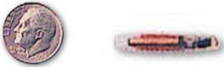
Figure 3. PIT tag (32 mm; 1.3”) shown with a dime coin for size comparison.
