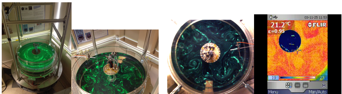
Figure 6: Examples of a baroclinic mode 1 (left hand side) and a baroclinic mode 4 (3 panels at the right) visualised via dye experiments and confirmed in infrared camera images.
