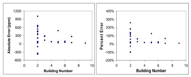
Figure 2. Absolute and percent errors from single point calibration checks of CO<sub>2</sub> sensors.
