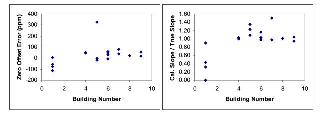
Figure 1. Zero offset errors and slopes from multipoint calibration checks of CO<sub>2</sub> sensors.
