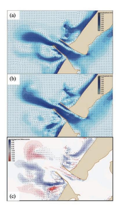
**Figure 6.** Velocity field at peak ebb tide (large waves, cross-jetty): (a) one-way; (b) two-way; (c) difference in current magnitude (two-way minus one-way; blue indicates higher speeds in the two-way model; red indicates higher speeds in the one-way model).
