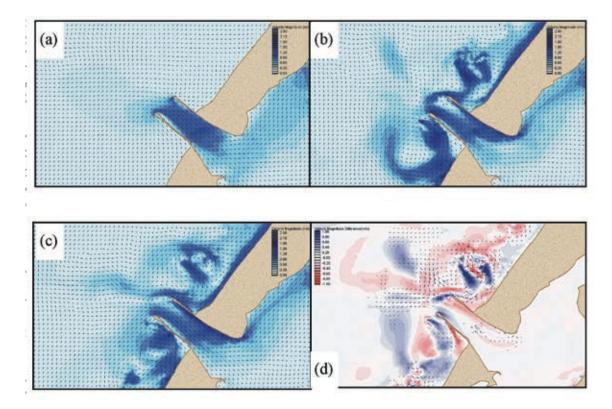
**Figure 10.** Velocity field at peak ebb tide for large waves, down-jetty: (a) uncoupled; (b) one-way; (c) two-way; (d) difference in current magnitude (two-way minus one-way; blue indicates higher speeds in the two-way model; red indicates higher speeds in the one-way model).
