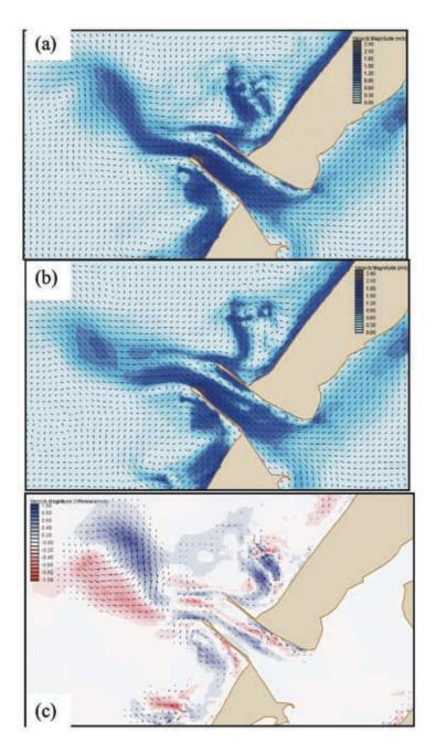
**Figure 5.** Velocity field at peak ebb tide for large waves, down-jetty: (a) one-way coupled; (b) two-way coupled; (c) difference in current magnitude (two-way minus one-way; blue and red indicate higher speeds in the two-way and one-way models, respectively).
