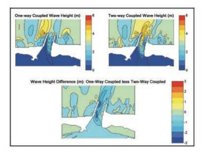
**Figure 8.** Comparison of wave-height fields for large, down-jetty waves at peak ebb. Two-way coupled solutions were more than 1.9 m higher over the channel shoal and more than 1.7 m higher in the navigation channel than one-way coupled solutions.
