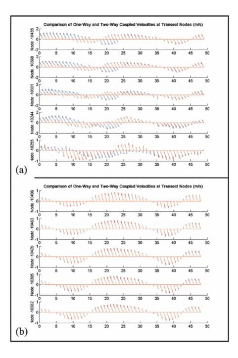
**Figure 13.** Comparison of half-hourly vector velocities along transect nodes for one-way (blue) and two-way (red) coupled model runs for large, down-jetty waves: (a) Transect 2; (b) Transect 3. Numbers along the x-axis denote semi-hourly time steps. The y-axis scale is in m/s.
