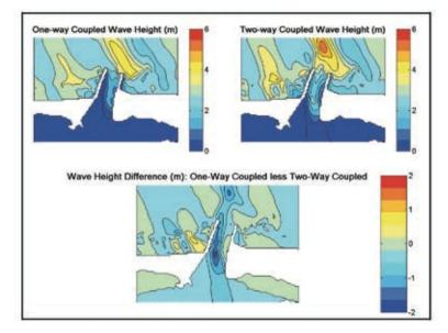
**Figure 9.** Comparison of wave-height fields for large, cross-jetty waves at peak ebb. Two-way coupled solutions were more than 1.9 m higher over the channel shoal and more than 1.7 m higher in the navigation channel than one-way coupled solutions.
