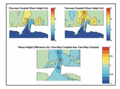
**Figure 7.** Comparison of wave-height fields for small, down-jetty waves at peak ebb. Two-way coupled solutions were more than 1.1 m higher over the channel shoal and more than 0.9 m higher in the navigation channel than one-way coupled solutions.
