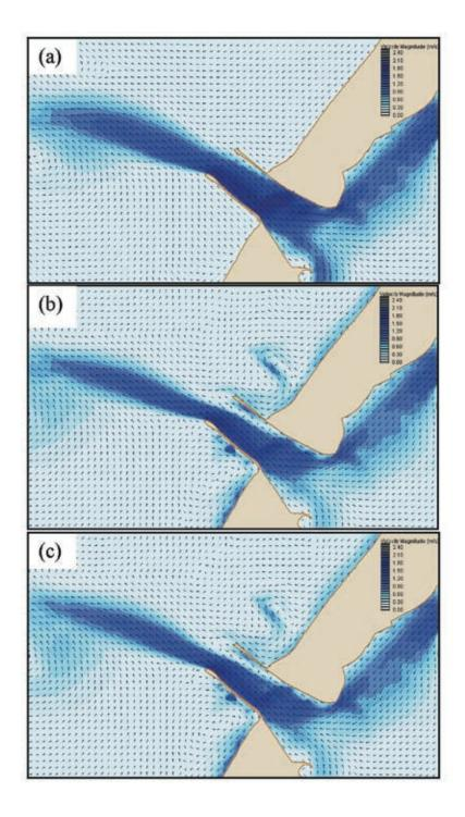
**Figure 4.** Velocity field at peak ebb tide for: (a) all uncoupled model runs; (b) small waves, down-jetty, one-way; (c) small waves, down-jetty, two-way. Color scale describes current magnitude; arrows identify current direction.
