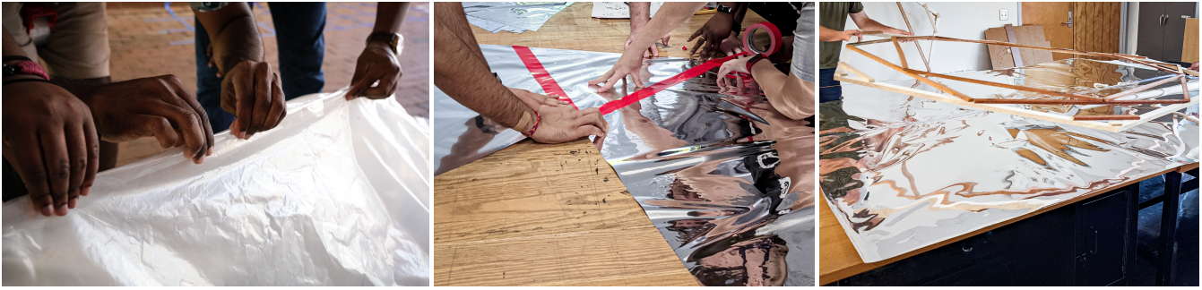
Figure 3: Fabrication: After 3D modeling shapes and ‘unwrapping’ 2D surfaces as patterns, shapes were cut out of sheet material using frames or other stencils (right) and required many hands to hold the pieces in place and tape along the seams (left, middle).
