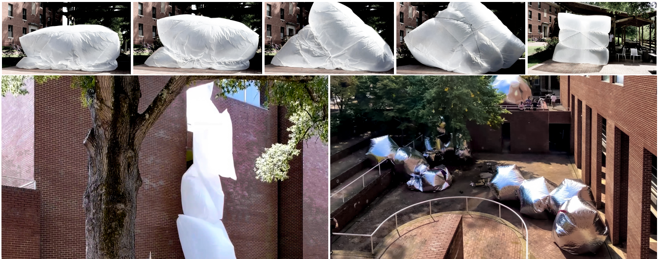
Figure 1: Iterations: Our iterative prototypes increased in scale and technical difficulty over time. (top row) One of the first inflatables we made, a 3m cube wrapped with cords shown inflating. When inflating up to size, inflatables tumble, writhe, and transform before settling into their equilibrium shape, gently swaying but stable. (middle) Several 3m square ‘pillows’ cascade down a building, glowing in the light and swaying in the breeze. (bottom) The assemblage of rounded foil forms felt like alien meteors that had recently fallen to earth, or monstrous dew drop pearls.
