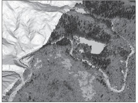
LIDAR'S VIEW OF THE ANGELO RESERVE — A SMALLER SECTION IN GREATER DETAIL — SHOWS INDIVIDUAL TREES. IMAGE COURTESY OF THE NATIONAL CENTER FOR EARTH-SURFACE DYNAMICS (NCED)
