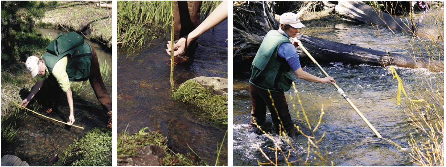
To estimate flow volume, Bobbette Jones, UC Davis graduate research assistant, measures the stream's: left , width; center , depth; and right , velocity. In this study, every cubic-foot-per-second increase in stream flow was associated with a 1.64°F decrease in daily maximum stream temperature.
