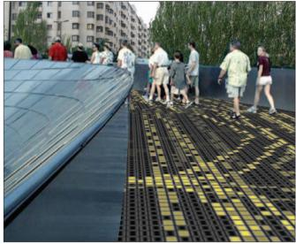
Above: Portillo: Memory pavement uses digitally responsive ground surfacing to record footfalls of pedestrians, displaying how pathways are reinforced by multiple trips. Luminescence accretes into lines and spaces: one passage would be invisible; multiple passages would be rewarded, encouraging pedestrians to examine pathways and try new ones. Images by Rajesh Kottamasu.
