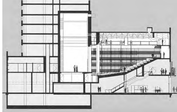
Theatre Row, section, showing weaving of multiple-theatre access lobby, upper-level theatre, and apartments into a complex site. Courtesy Hardy Holzman Pfeiffer
