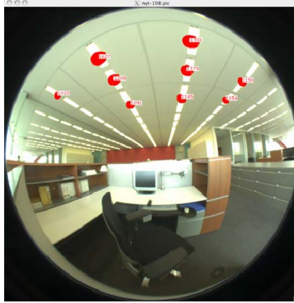
Fig. 6 Glare analysis of a HDR photograph from a workstation on the Northwest part of the mockup. (Multiple exposure images are taken on 10/27/2004 between 13:28:53 – 13:29:50; aperture size of f/4; shutter speed between 1 - 1/1000 sec)
