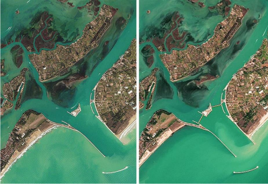
Figure 33-9: Satellite imagery of the Venice floodgates open, on November 4, 2021 (left), and closed, on November 6, 2021 (right).
