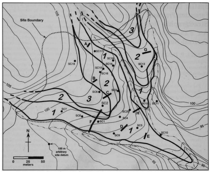
Figure 1. Geomorphic surface map of 26EK5040 showing terraces (1,2, and 3), backhoe trenches (A-H), and soil core locations (SC1-SC20); contour interval is 1 meter. (after Ataman et al. 1995).
