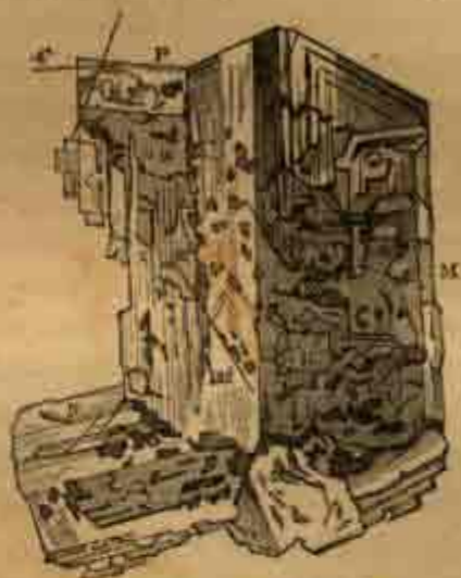
FIG. 32.—Andesite of Camiguin. Section of plagioclase, Baveno, albite, and pericline twins. \frac{1}{2} crossed nicole.
