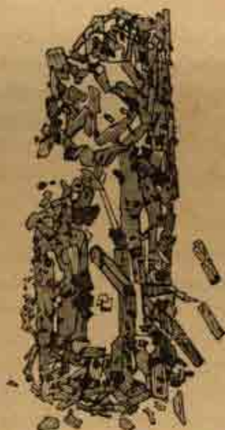
FIG. 21.—Augitic trachyte from Royal Sound. Small grouped crystals of augite, imitating as a whole the form of a hornblende crystal, whose place they fill. This replacement of hornblende by augite has been accompanied by the formation of numerous grains of magnetite, and in the centre of the group of augites a small brownish pleochroic remnant of hornblende may be seen. Usually, as in the drawing, this mineral has quite gone, zeolites filling the interstices between the augite microliths. \times , crossed nicols.
