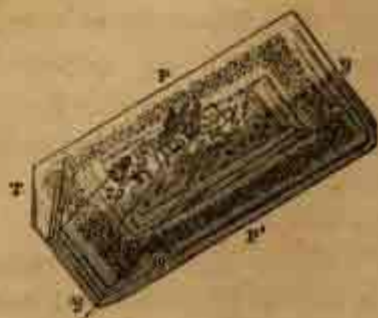
FIG. 34.—Andesite of Camiguin. Section of plagioclase following M , pericline twin, \frac{1}{2} crossed nicole.
