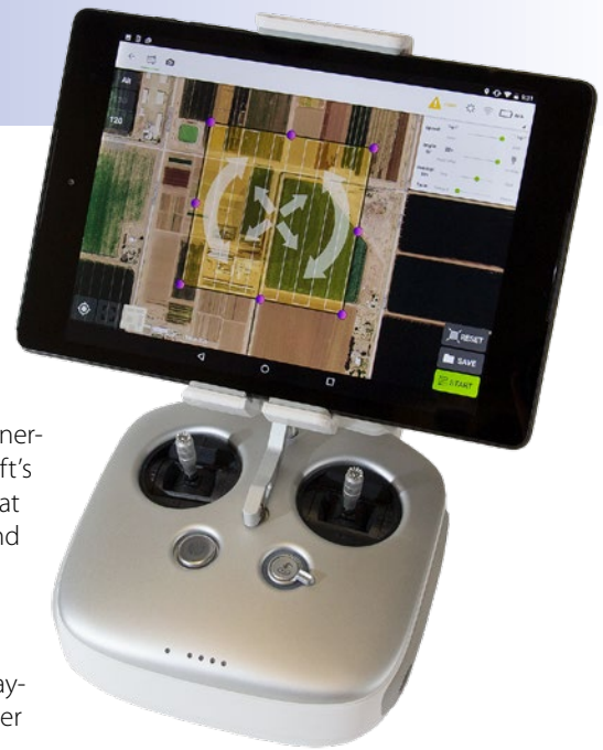
Controller for a DJI Inspire 1 drone. The attached tablet shows an in-flight view and other information.
