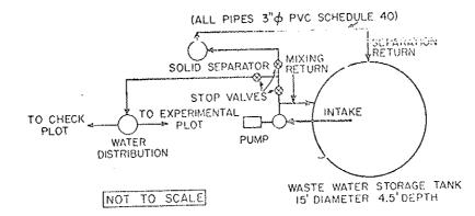
Fig. 4. Wastewater storage, solid separation and delivery system.
