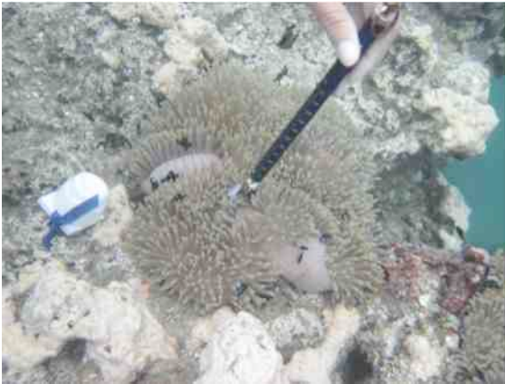
Fig. 10. The measurement of tentacle adhesiveness. A spring scale was used to calculate the force, frozen shrimp was used as bait for attachment. Picture by C. Lewis.
