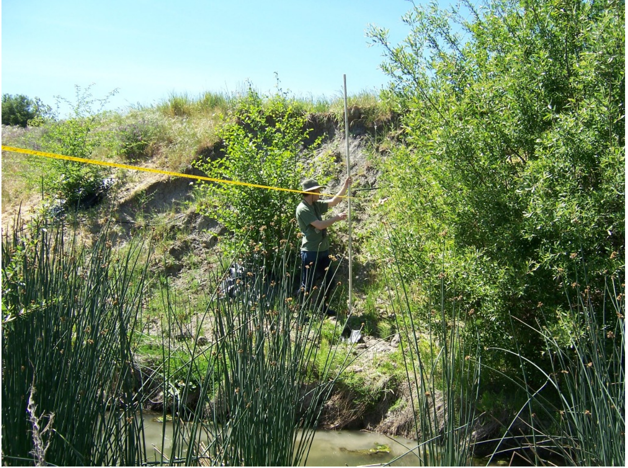
Figure 3: Measuring cross-sectional area of the stream at Alamo Creek. 4/19/2008
