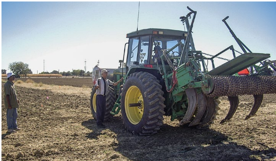
Trial results suggest that GPS-controlled spot fumigation has the potential to reduce fumigant use. Above, testing the fumigant applicator at UC Davis.
