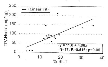
Figure 1. Relationship of total PAHs normalized to dry weight (TPAHsdw) or to sediment organic carbon (TPAHsoc) to the percentage of silt in sediments in Hoffman Marsh in 1993-94. Note the linear and statistically significant relationship of the PAHs to silt and that the most silty (small particle) sediments contained the most PAHs.
