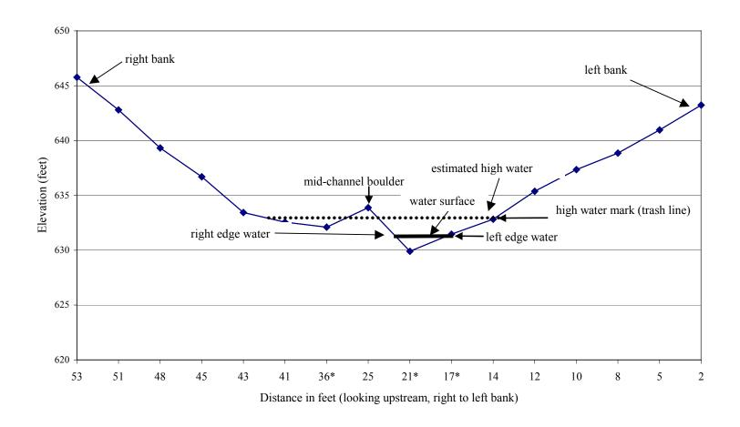
Figure 7. Lower Reach Cross-Section
