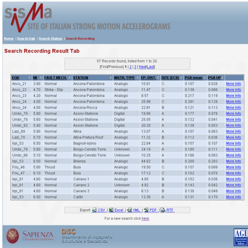
Figure 3.9. Table listing records having PGA=0.1-0.3g on type C soil according to EC8
