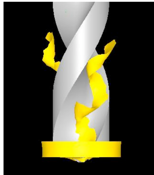
Figure 7: DEFORM simulation showing the formation of a burr in a flat exit surface
