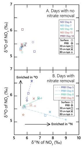
Fig. 4. On days with nitrate removal, residual subsurface nitrate is enriched in  $\delta^{15}N$  and  $\delta^{18}O$ , consistent with denitrification. A.  $\delta^{15}N$  and  $\delta^{18}O$  for five days with no nitrate removal. B.  $\delta^{15}N$  and  $\delta^{18}O$  for four days with nitrate removal; dashed lines connect surface and deepest samples.
