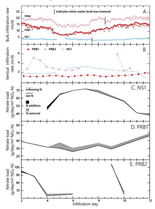
**Fig. 2. More nitrate was removed below a PRB than in native soil.** A. Bulk infiltration rates. B. Vertical infiltration rates. C,D,E. Inflowing nitrate load (*dashed lines*) and net nitrate load at deepest subsurface sample (*solid lines*). *Grey shading* indicates nitrate removal; *black shading* indicates nitrate addition. Data gaps during test PRB2 are times when vertical infiltration was too rapid to resolve accurately (see Supporting Information).
