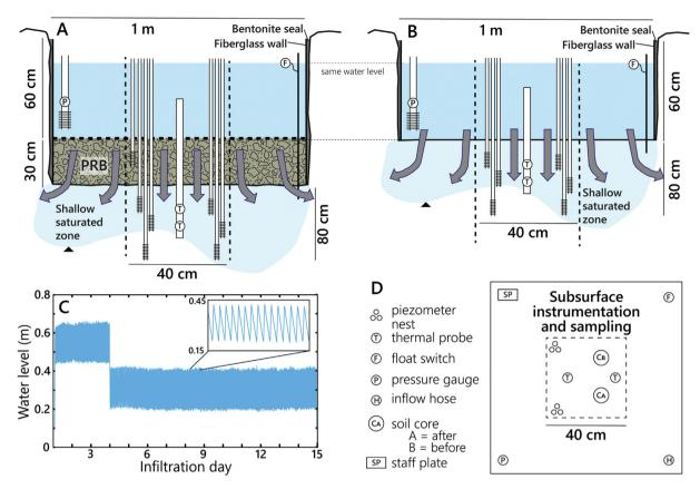
**Fig. 1. Experimental design.** A. Cross section of PRB experimental plot, showing float valve (*F*), thermal sensors (*T*), pressure gauge (*P*), and piezometers. Black triangle shows the inverted water table created by infiltration. B. Cross section of native soil plot. C. Water level over time during test PRB1; inset highlights three hours of infiltration. D. Plan view of instrumented experimental plots, with central instrumented area delineated.
