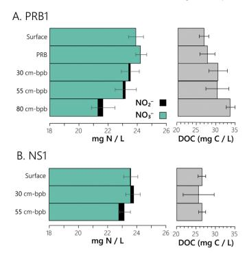
Fig. 3. [NO<sub>3</sub>-N] decreased and [DOC] increased with depth below the PRB; changes were less consistent in native soil. Average [NO<sub>3</sub>-N] and [NO<sub>2</sub>-N] (left) and [DOC] (right) with depth over days 5–12 from tests PRB1 (A) and NS1 (B). Error bars show one standard deviation for all samples.
