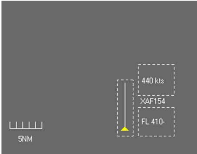
Figure 1: Screenshot of an aircraft cruising at the constant altitude of FL 410. Its speed is 440 kts. A scale representing 5NM was presented at the bottom left of the display. Here, dashed lines represent the areas of interest (AOI) used to compute eye fixations, but they were not visible by participants.
