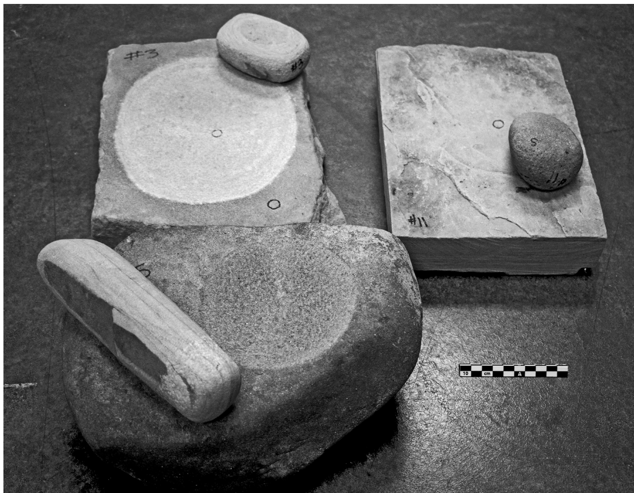
Figure 9. Three sets of experimental sandstone milling tools.
