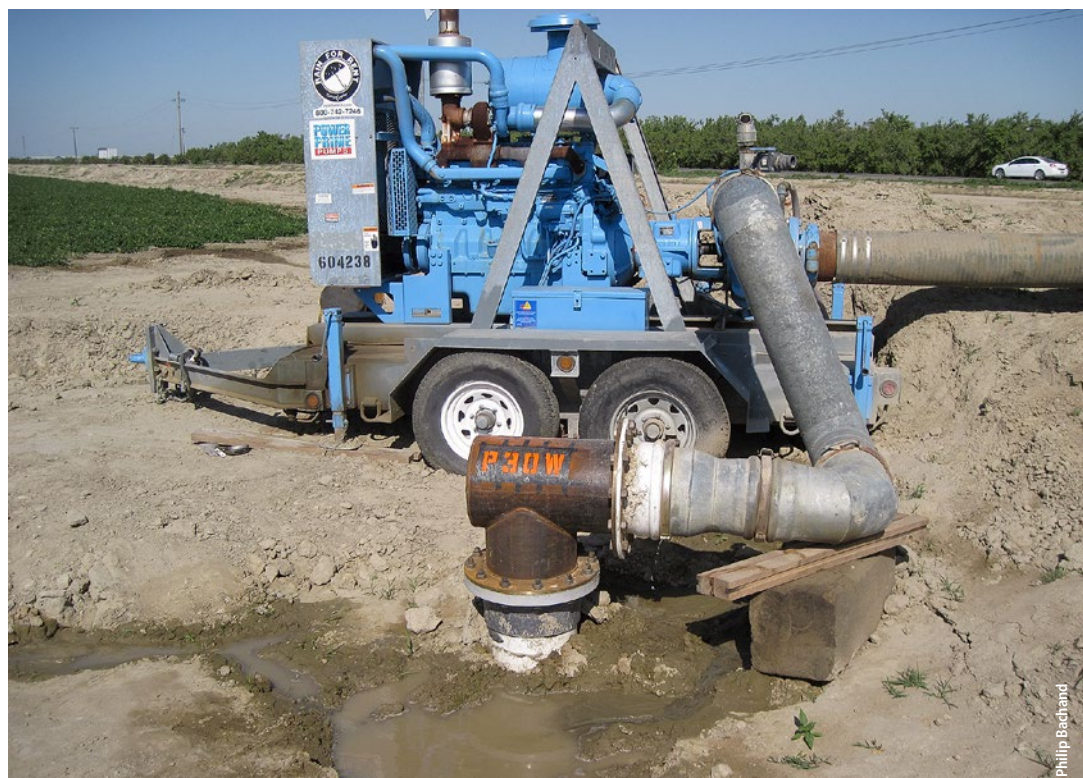
Pumps and engines were connected to piping to pull floodwater onto agricultural fields from the diversion canal on the James Bypass.
