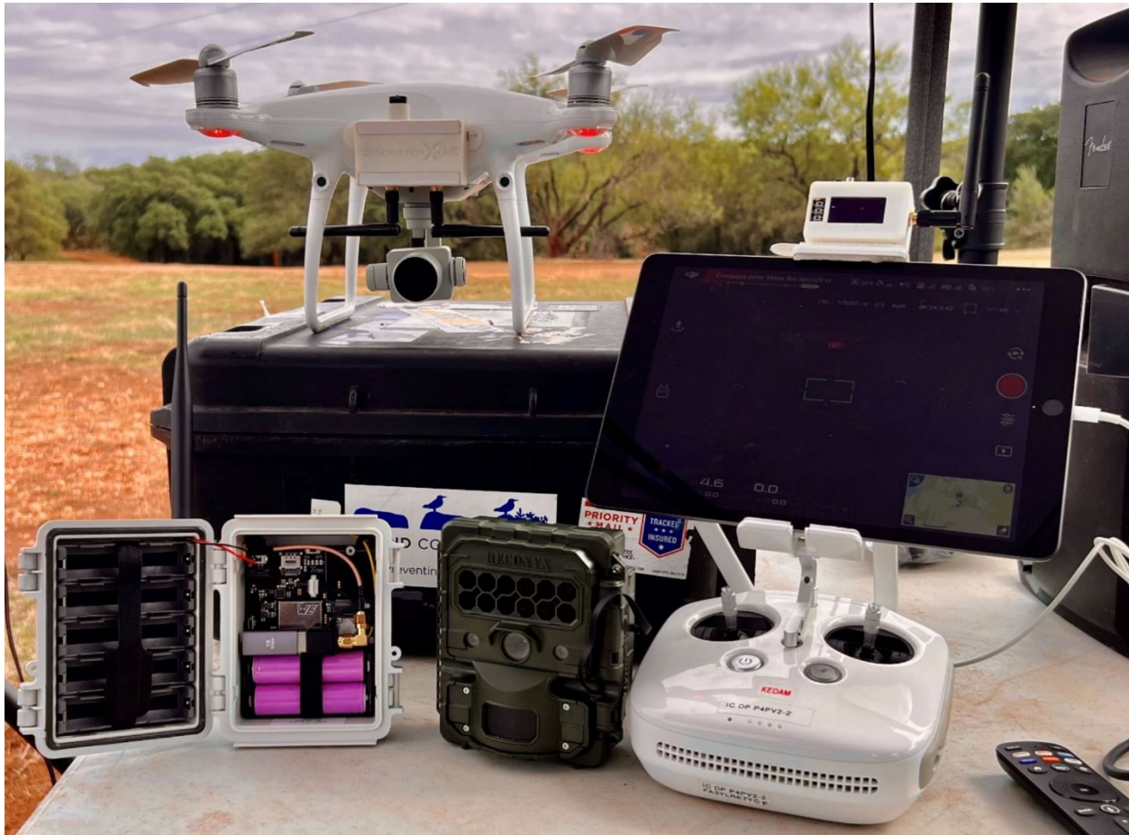
Figure 1. The full prototype solution at the end of AUL 5, including a Sentinel drone payload attached to DJI Phantom 4 with receiver mounted to the drone controller. Open Sentinel device next to Reconyx camera trap.
