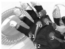
Figure 2: Layout of the 12 force sensors on the fingertips and palm.
