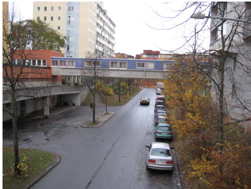
Fig. 3. The Million Homes Program was inspired by modernist ideas in architecture, which, amongst other things, found expression in the separation of roads for motorized vehicles and roads for pedestrian use. Photo credit: J. Kustermans.
